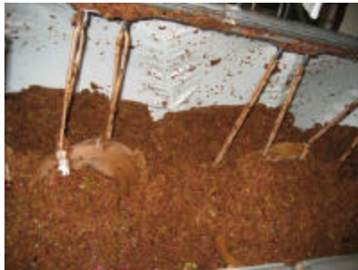
Drainage Loops in the Middle of Mash at the End of the Extraction (dry pomace)
